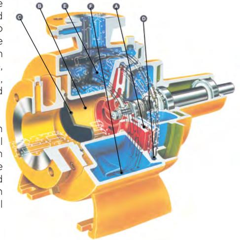
If for some reason, air penetrates into the suction pipe and the pump stops pumping, the priming process starts again and described above, as continues until normal pumping has been resumed.
