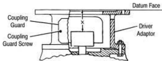
2. Determine the end gap (the distance between each coupling hub) for the size of coupling provided. Refer to the Coupling Specifications tables in the Specifications section of this manual for specific measurements.
