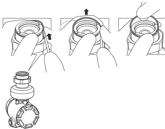
2. Replace the transmitter head nut.
