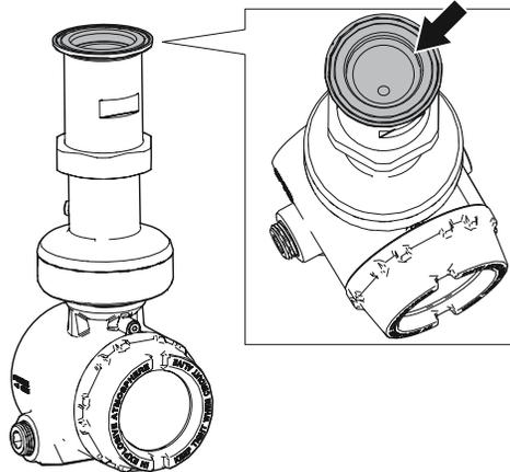
2. Verify the O-ring on the PTFE sealing is in place.
