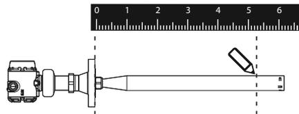
3. Cut the antenna at the marking.
