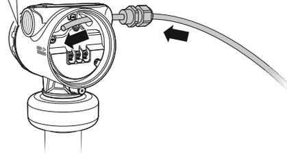
5. Connect the cable wires.
