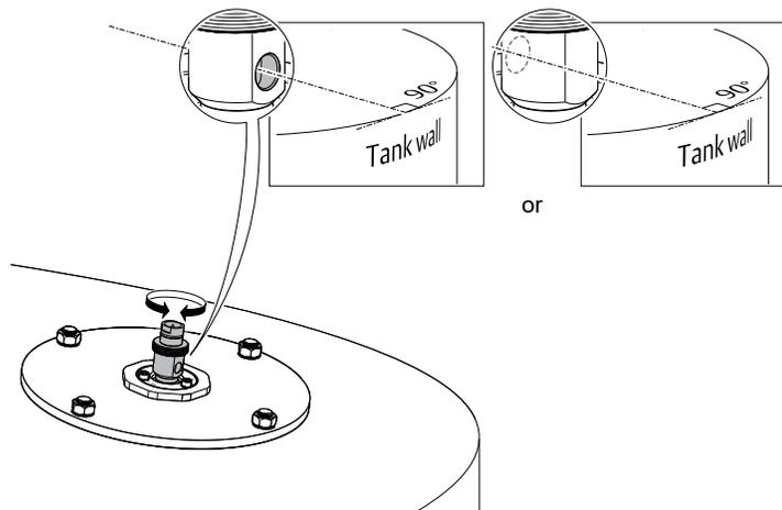
3. Place the supplied circular level on top of the antenna assembly.
