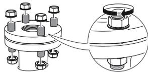
4. Apply anti-seize paste or PTFE tape on threads according to your site procedures.
