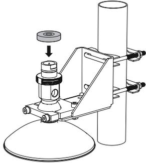
4. Adjust the inclination of the antenna.
