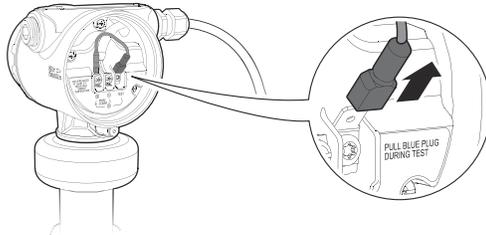
4. Connect the ampere meter leads to the terminals labeled "+" and "TEST".
