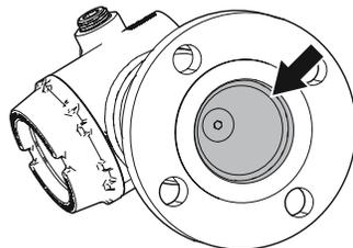
2. Verify the O-ring on the PTFE sealing is in place.
