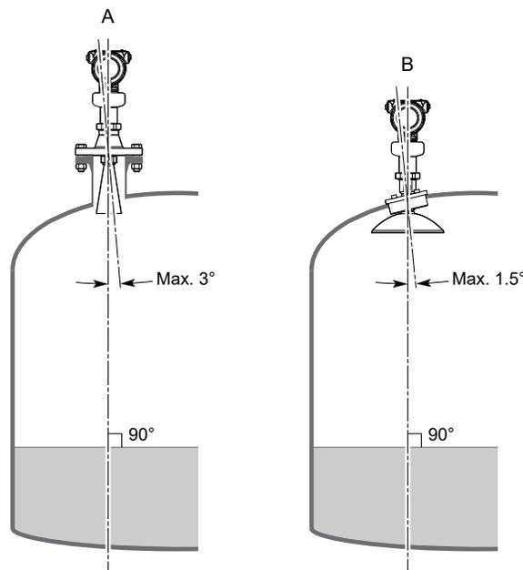
A. Cone antenna/process seal antenna
