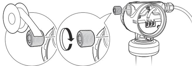
9. Attach and tighten the cover.
