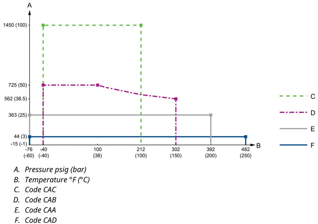
Figure A-3: Cone Antenna (PEEK Seal)
