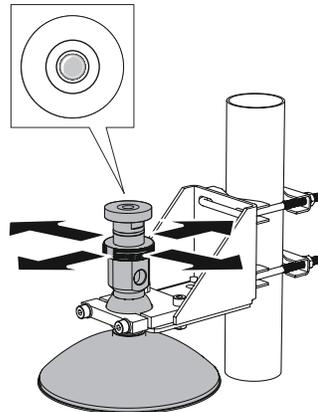
5. Gradually tighten the two M8 screws.
