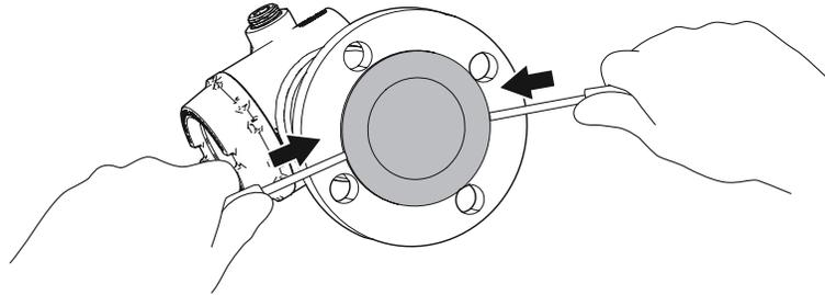
2. Gently push the screwdriver handles forward until the PTFE sealing pops out.
